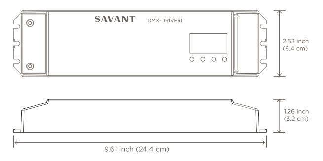
HELPFUL! To mount the driver to a wall or similar, choose any of the three fixing screw holes located on either end of the driver.
